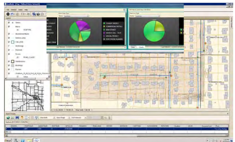
Intranet GIS data Browser Viewing Wastewater Data with an As-Built Back Drop
